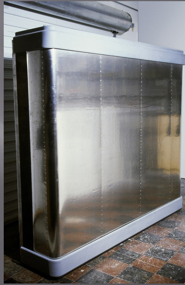
Faraday cage using rolling way cover with copper contact strip
