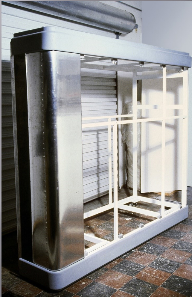
Faraday cage using rolling way cover with copper contact strip
